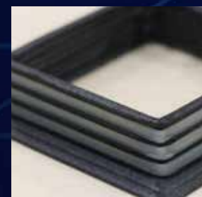
3D combined extrusion printing of pellet and filament
